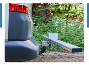
Mounted at the towing hitch, sensor values are collected and the road quality of unpaved, single lane roads gets assesd. Ultrasonic sensors (cross section scan of a road segment) acceleration sensors to assess the longitudinal roughness and a GPS sensor for locatiion.
