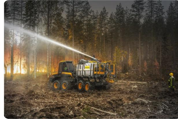
*PONSSE is introducing firefighting equipment to be installed in the load spaces of forwarders for extinguishing wildfires.*
