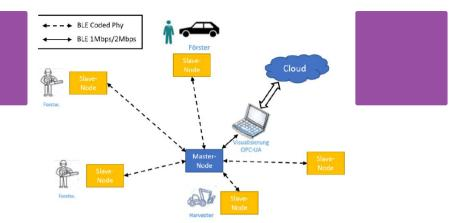
Improvement of work safety through a new IT solution. A sensor node network connects to anyone involved (carrying such a node) and provides information about current danger situation over license-free band using Bluetooth low energy (BLE).
