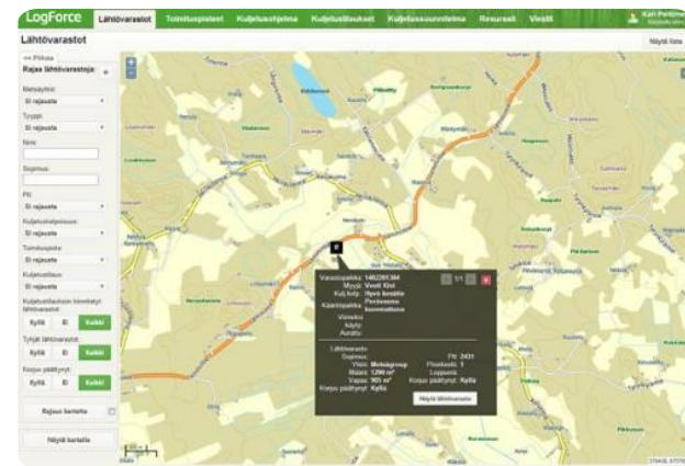
*CFLogistics (LogForce) is used by both forest companies and contractors. The planner can ensure that requested amounts of wood are transported to the delivery destinations. Also, the driver has real-time information on what is supposed to be delivered from where and to where.*
