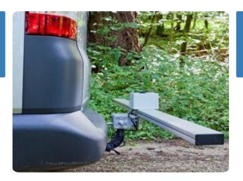
Mounted at the towing hitch, sensor values are collected and the road quality of unpaved, single lane roads gets assesd. Ultrasonic sensors (cross section scan of a road segment) acceleration sensors to assess the longitudinal roughness and a GPS sensor for location.
