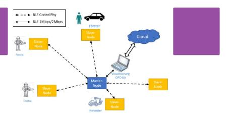
Improvement of work safety through a new IT solution. A sensor node network connects to anyone involved (carrying such a node) and provides information about current danger situation over license-free band using Bluetooth low energy (BLE).
