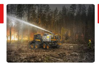
PONSEE is introducing firefighting equipment to be installed in the load spaces of forwarders for extinguishing wildfires.
