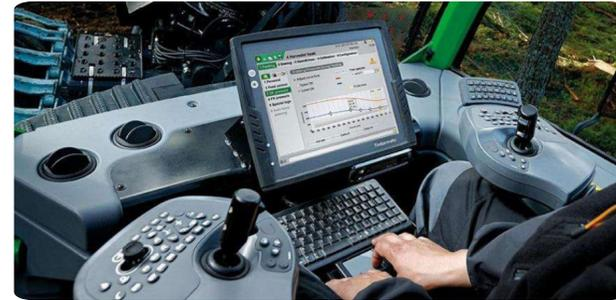
*Machine control systems and sensor technology compile directed feedback to guide the operator towards more balanced working methods and techniques.*
