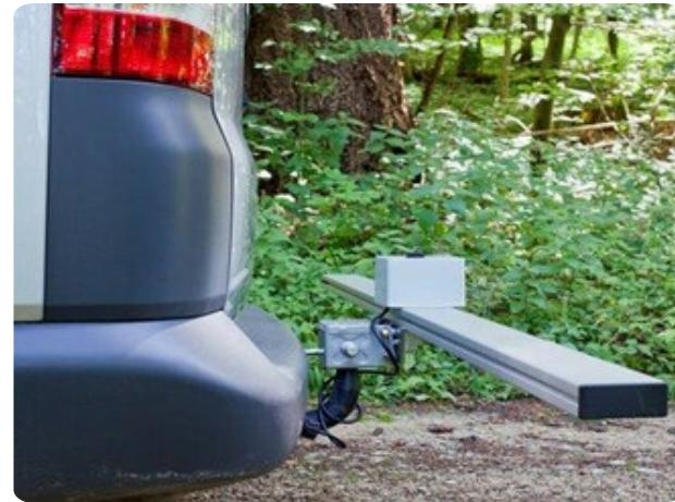
*Mounted at the towing hitch, sensor values are collected and the road quality of unpaved, single lane roads gets assessed. Ultrasonic sensors (cross section scan of a road segment) acceleration sensors to assess the longitudinal roughness and a GPS sensor for location.*
