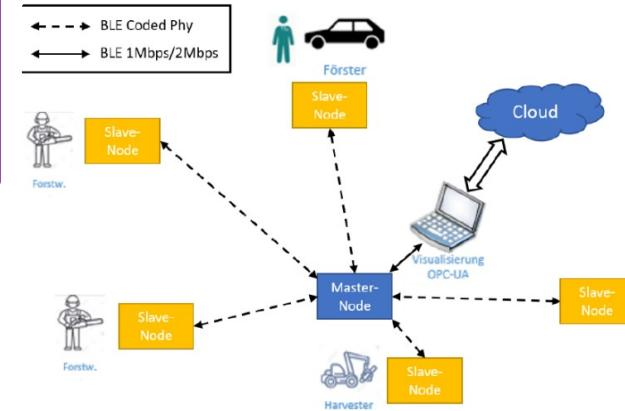
*Improvement of work safety through a new IT solution. A sensor node network connects to anyone involved (carrying such a node) and provides information about current danger situation over license-free band using Bluetooth low energy (BLE).*
