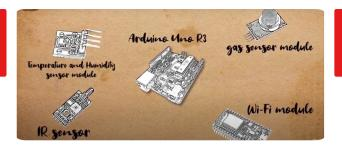
DecectIT is forest fire detection device which detects fire by using different sensors and sends nottification to the application.
