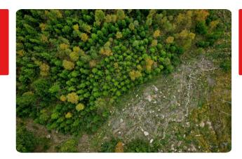
Precision forestry service that with the help of RGB and multispectral images from drones, airplanes, helicopters or satellites can detect bark beetle infected or stressed trees.
