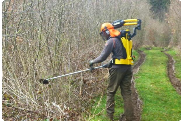
*The Extrafor project aims to reduce the drudgery of logging by creating an exoskeleton adapted to the needs of manual logging.*
